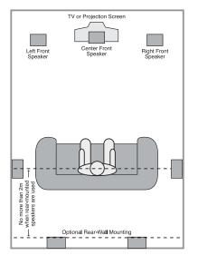
*B)* The distance between the left and right speakers should be equal to the distance from the seating position to the viewing screen. You may also experiment with placing the left and right speakers slightly forward of the center speaker. Rear speaker mounting is an alternate location for 5.1 systems.
